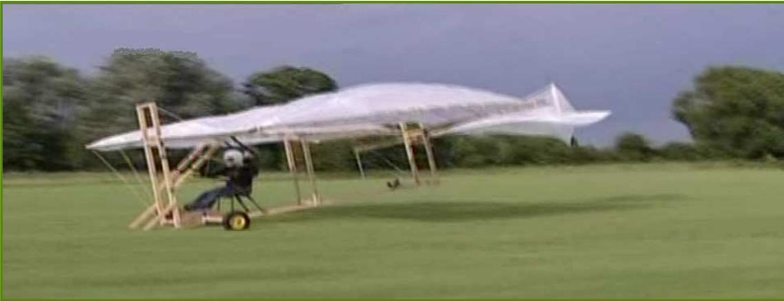
Clearly the authentic Cayley aerofoil was generating lots of lift and the rear end of the machine was nicely airborne, unfortunately causing the nose to dig into the ground, suggesting the machine's centre-of-gravity was too far forward. Some 'empirical redesign' (moving the pilot's seat further back...) and further testing failed to achieve a sufficient improvement; the front end remained stubbornly grounded.
